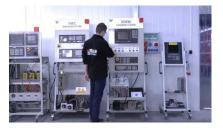
We have test stands developed by us, thanks to which we check whether the device is operational. They make sure that MEAN WELL SDR-480-48 is repaired.
